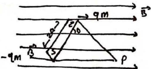
The force acting on the south pole is towards left. The force acting on the north pole is towards right.
