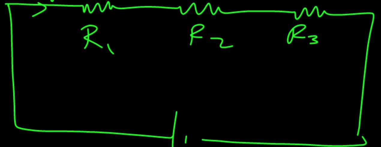
$$R_{eq} = R_1 + R_2 + R_3$$
