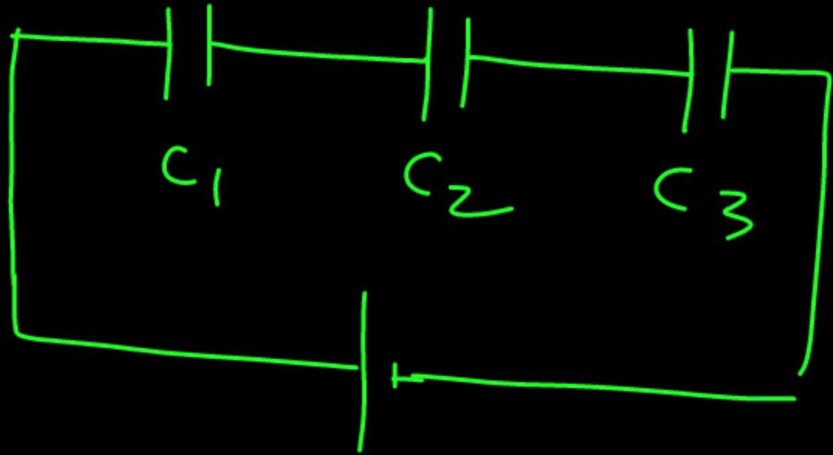
$$\frac{1}{C_e} = \frac{1}{C_1} + \frac{1}{C_2} + \frac{1}{C_3}$$
