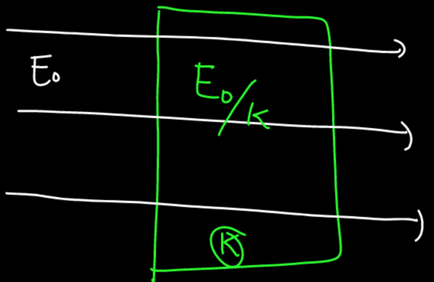
1. Parallel plate capacitor with completely filled dielectric
